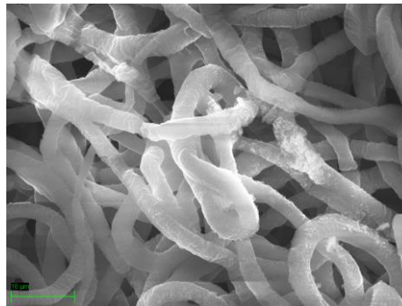
Fig .4 HRSEM picture of BEC 1 as-electrospun(after cryogenic applications ) fibers
