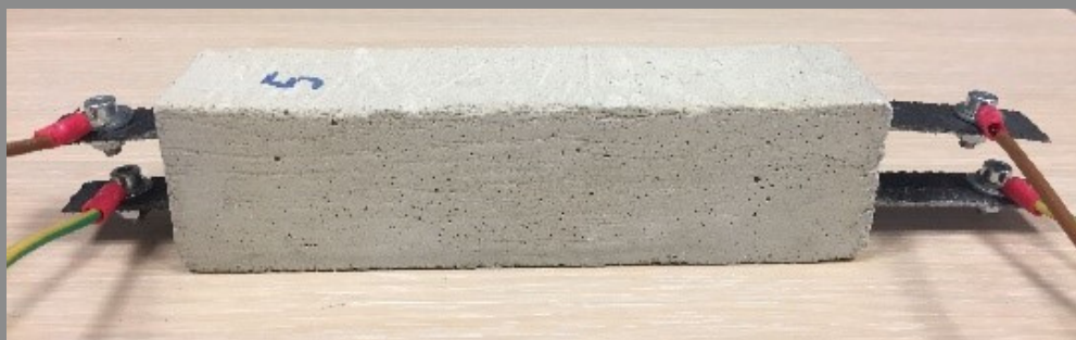
Figure 12 – Textiles with sensing carbon coatings embedded in concrete to detect load changes and prevent damages
