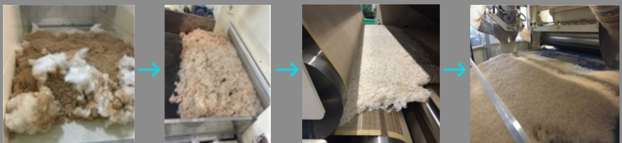
Figure 22 - Textile waste recycling process 18
