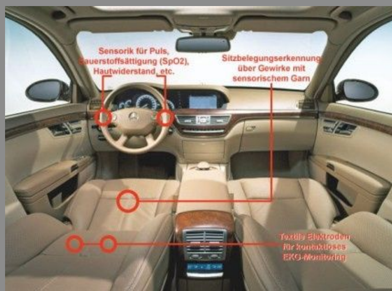
Figure 9 - Concept for textile seat occupation sensor realized by crimp interconnection (INSISTEX project)
